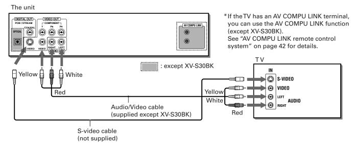
Connect the unit to a TV equipped with stereo audio input and video input jacks using the supplied audio/video cables.
